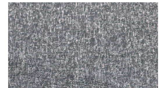
Ne45 woven Sample Cover: 100% Lyocell Core yarn: 30d polyester Only the cover fiber is dyed.
