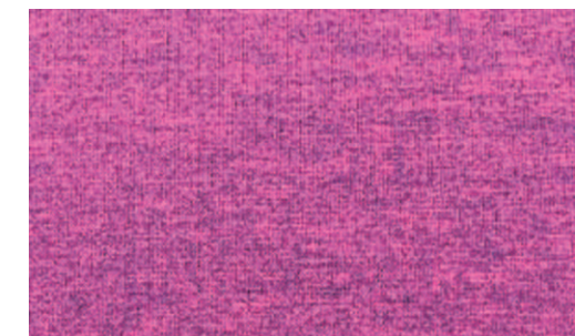
Ne30 Knit Sample Cover: 100% rayon Core yarn: 70d polyester Only the cover fiber is dyed.
